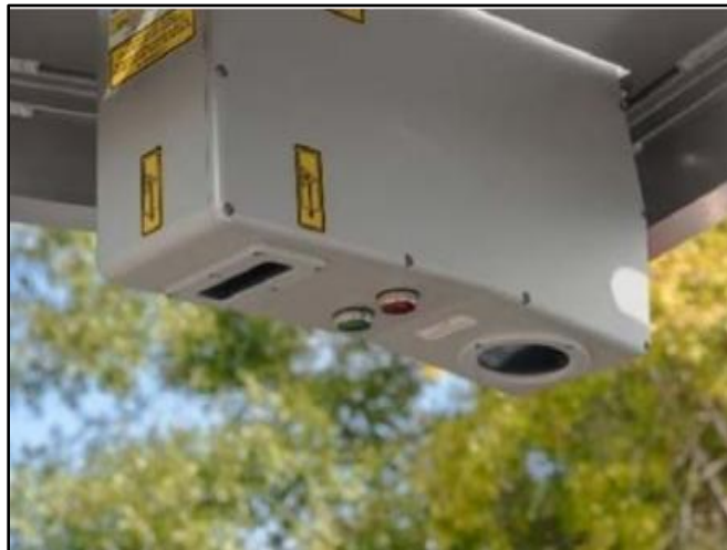
Figure 5: LCMS-2 Pavement Imaging System
