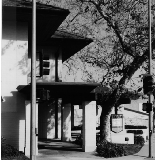
Entry arcades and porches may be used in front of or alongside buildings, also screening parking from street view.
